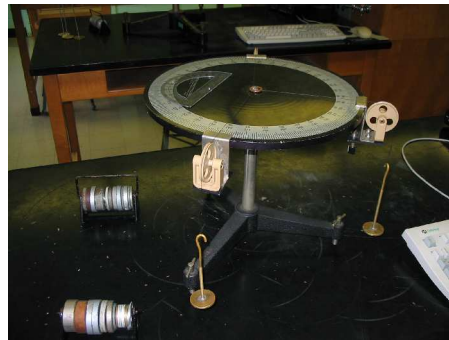
Figure 3.3: The force table used for the experiment
