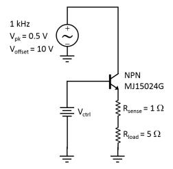
This circuit is a basic current controller. The current comes from the AC source, which we are using as a constant voltage source (with voltage  $V_{offset}$ ) with some sinusoidal "noise" at 1 kHz and amplitude  $V_{pk}$ .
