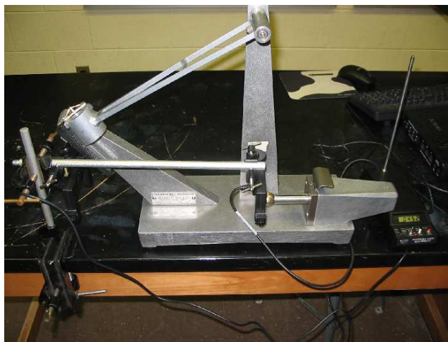
Figure 4.2: The ballistic pendulum with the pendulum on the ratchet mechanism which prevents the pendulum ring from falling from its maximum height.
