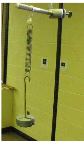
Figure 3.1: Basic apparatus for the mass on a string.
