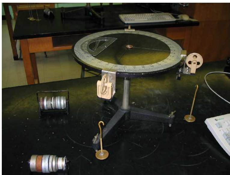
Figure 1.1: The photograph shows the force table with the the pulleys, weight hangers and slotted weights.
