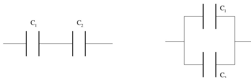
Figure 6.2: Series (left) and parallel (right) capacitors.
