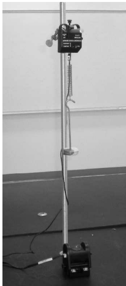
Figure 9.1: This photograph shows the harmonic motion setup. The force sensor and spring are at the top. The weight hanger should be placed directly over the motion sensor.
