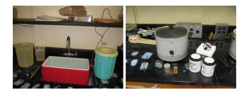
Figure 3.1: Equipment for this lab including the Styrofoam calorimeter, metal samples, water baths and digital thermometer
