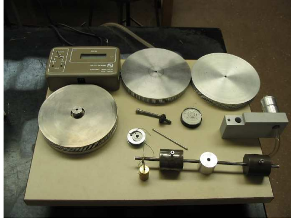
Figure 9.1: The rotational motion apparatus. The two steel and one aluminum disk are shown along with the bobbin, barbell and other items
