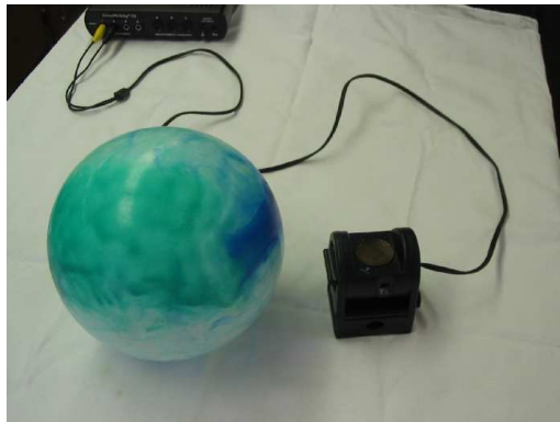
Figure 7.5: Ball and motion detector used in this lab.
