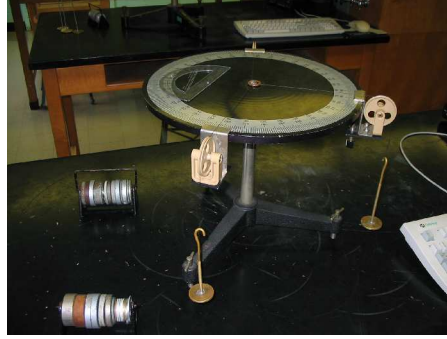
Figure 3.3: The force table used for the experiment
