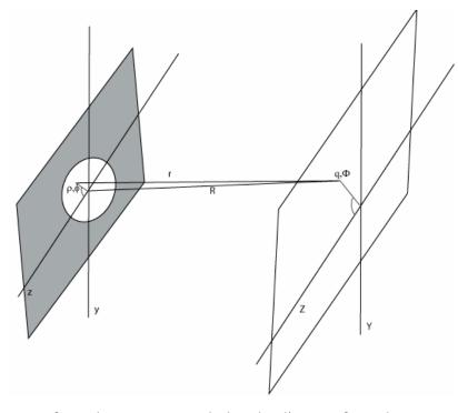
To find the amplitude of the electromagnetic field passed through a circular aperture of radius *a* we need to add contributions from all points of the aperture taking into account the relative phase difference due to difference in path length from different aperture points to a point on the screen. Polar coordinates  $\rho$  and  $\phi$  describe a point on the aperture, and we will be interested in the light intensity. We will be interested in the diffraction pattern far
