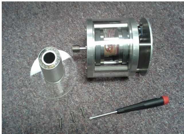
Figure 3.15 VT6S Velocity Transducer showing (left) source shield off and gamma source mounted on motor shaft and (right) source shield mounted on transducer. Visible through the transparent case are the magnets for the drive coil and the velocity pick-up coil.
