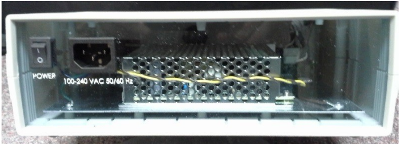
Figure 3.18 W304S Rear View showing the 100 – 240 VAC, 50 – 60 Hz line power connector with ON/OFF rocker switch.
