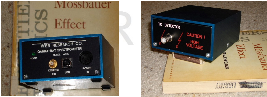
Figure 3.7 Front and Rear views of the W202S Gamma-ray Spectrometer. Case dimensions are 5 cm x 10 cm x 12 cm.
