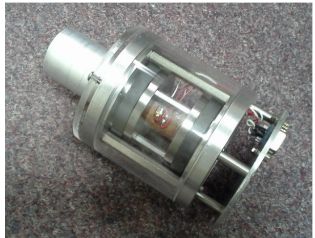
Figure 3.15 VT6S Velocity Transducer showing (left) source shield off and gamma source mounted on motor shaft and (right) source shield mounted on transducer. Visible through the transparent case are the magnets for the drive coil and the velocity pick-up coil.
