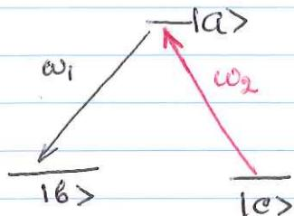
Two-photon process: one photon of  $\omega_1$  is emitted, one photon of  $\omega_2$  is absorbed
