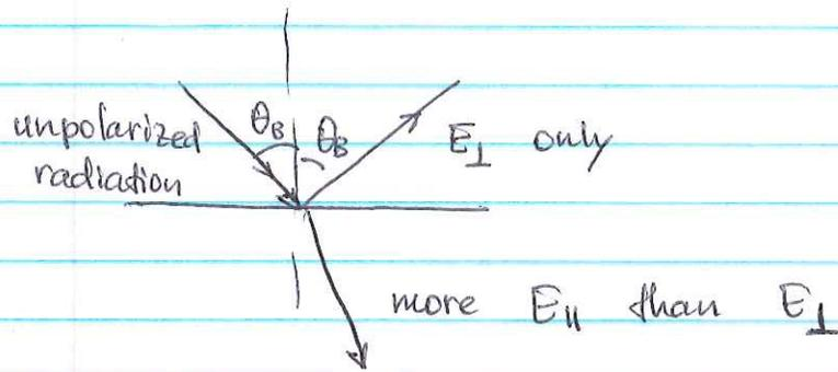
This is the principle of polarizing sunglasses: sunlight reflected off the road is partially polarized, so if the sunglasses ~~do~~ block this polarization, they reduce the effect of glare.
