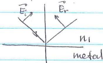
$$\underbrace{E_i \cos \theta_i - E_r \cos \theta_r}_{\text{air side}} = 0_{\text{metal side}}$$
