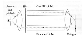
through separate hollow airtight arms of length *L* each with glass entry and exit windows. The separate beams are brought together by a lens with fringes appearing in the image plane. Both arms are initially evacuated and gas is introduced slowly into one arm. This causes the fringes to move across the field of view; up or down in the diagram. If *m* fringes pass through the center of the field while the gas is entering,
