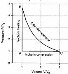
The Lenoir cycle is an idealized thermodynamic cycle often used to model a pulse-jet engine. The cycle consists of three stages: first, the gas is heated at constant volume, then it undergoes adiabatic expansion, and finally the exhaust at constant pressure. Shown below is an example of Lenoir cycle in which one mole of an ideal diatomic gas  $(\gamma=C_P/C_V=7/5)$  is taken though the cycle. In the starting point A the volume of the gas is V<sub>0</sub>, and its pressure is P<sub>0</sub>.
