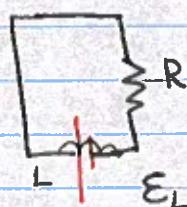
$$\begin{aligned} E_L - IR &= 0 \\ -L \frac{dI}{dt} - IR &= 0 \end{aligned}$$
