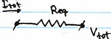
$$I_{tot} = \frac{V_{tot}}{R_{eq}} = \frac{V_{tot}}{R_1} + \frac{V_{tot}}{R_2}$$
