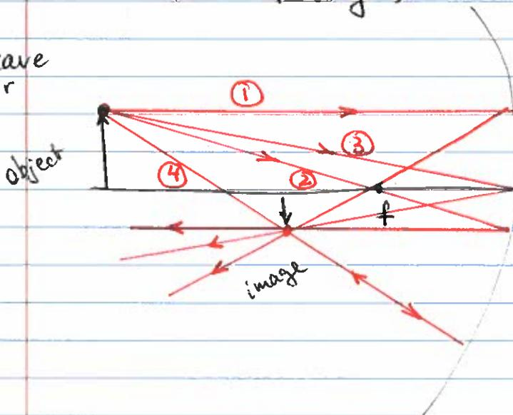
① Parallel to optical axis → ~~cross~~ pass through focal point
