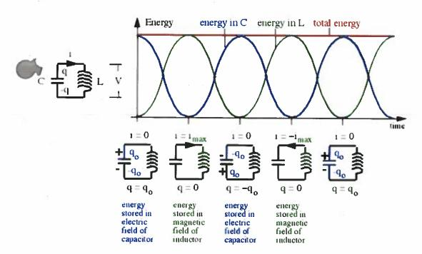
What if we add a resistance?  $\frac{Q}{C} = IR = L \frac{dI}{dt} = 0 \qquad I = -\frac{dQ}{dt}$   $\frac{d^2Q}{dt^2} + \frac{R}{L} \frac{dQ}{dt} + \frac{Q}{LC} = 0$  $\frac{d^2x^2}{m} + \frac{d^2x}{dt} + kx = 0$ oscillator with losses T(+) A decaying 0 scillastons If R is large, it discipates energy too quickly, no oscillations can happen If R is not too large R<- 4L/C
