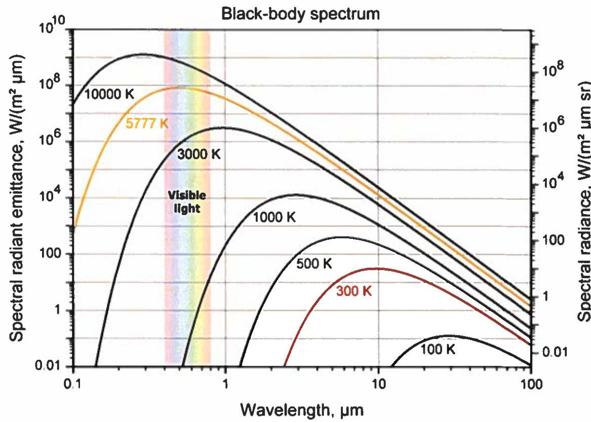
Radiation - energy is transferred through emission and absorption of electro-magnetic waves. Does not require any material contact b/w two objects
