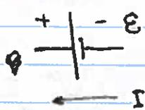
A battery provides an emf (constant voltage) to move charges in a closed loop
