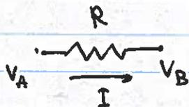
$$V_B - V_A = -IR \quad \text{voltage drop}$$
