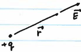
Electric field of a point charge
