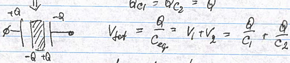
$$C_{\text{eq}} = \frac{1}{C_1} + \frac{1}{C_2} + \dots$$
