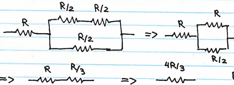
$$I_{\text{battery}} = \frac{E}{R_{\text{eq}}} = \frac{3E}{4R}$$
