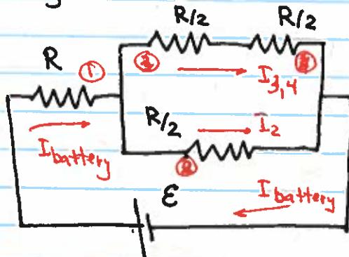
1. Let's find  $I_{\text{battery}}$  by calculating the equivalent resistance
