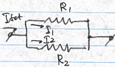
$$V_{R_1} = V_{R_2} = V$$
