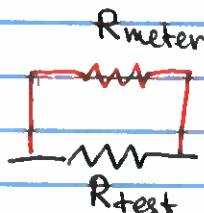
$$\frac{1}{R_{eq}} = \frac{1}{R_{test}} + \frac{1}{R_m}$$
