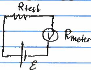
$$I = \frac{E}{R_{test} + R_{meter}} \rightarrow 0 \text{ if } R_{meter} \text{ is large}$$
