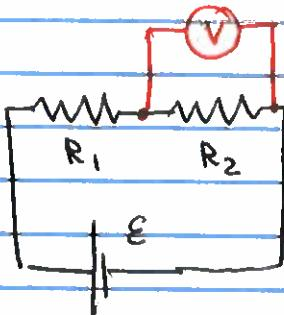
To measure the voltage drop across, say,  $R_2$  it must be connected in parallel with  $R_2$
