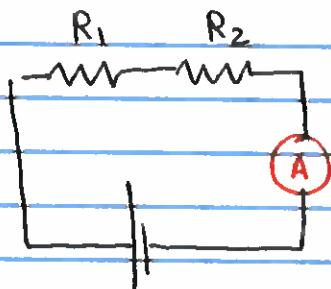
To measure the current through the circuit, the meter should be inserted into the loop
