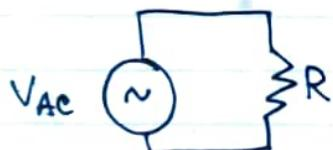
$$V_{AC}(t) = V_{max} \cos \omega t$$
