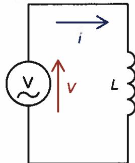
$$i(t) = \frac{V_{max}}{\omega L} \sin \left( \omega t - \frac{\pi}{2} \right)$$
