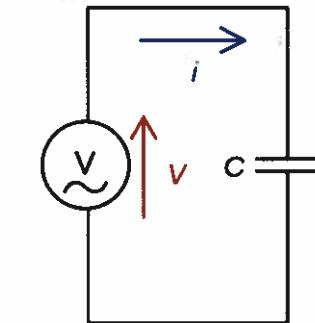
$$i(t) = \omega C V_{max} \sin \left( \omega t + \frac{\pi}{2} \right)$$
