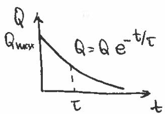
$$I(t) = \left| \frac{dQ}{dt} \right| = \left| -\frac{Q_{\max}}{RC} \right| e^{-t/RC} = I_{\max} e^{-t/RC}$$
