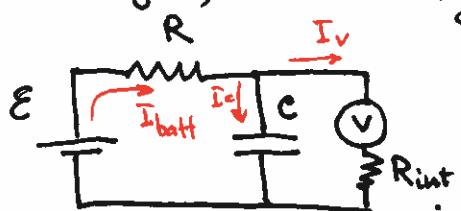
The voltmeter will show the voltage drop across the capacitor
