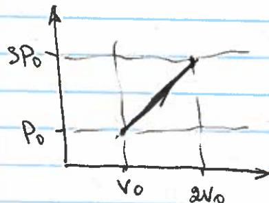
Equation: slope =  $\frac{\Delta P}{\Delta V} = \frac{2P_0}{V_0}$
