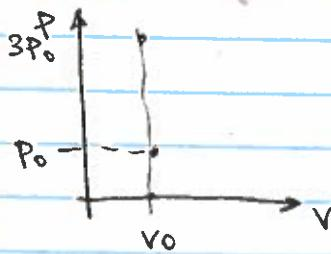
3. Temperature is constant  $T = \text{const}$  (isothermal)
