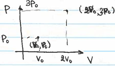
$$\text{Initial point } (P_0, V_0) \Rightarrow T_{\text{ini}} = \frac{P_0 V_0}{n R}$$
