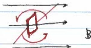
Electric turbine - rotating loop in constant magnetic field
