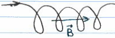
If a current through the solenoid changes,  $\vec{B}$  is changing  $\rightarrow$  EMF is induced in the coil (self-inductance)
