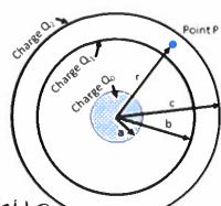
b) If the inner sphere is made of a conductor, find the value of the electric field everywhere. Make sure to define it in all four regions: r < a, a < r < b, b < a < c, and r > c.
