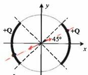
In the center E=0, since each section of the charge are produ has an opposite symmetrie section, so that their contributions to the electric field compensate each other.
