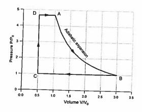
In 1859, Scottish engineer William John Macquorn Rankine proposed a cycle that became the foundation for modern heat engine and steam engine theory. The diagram shows a simplified Rankine cycle, in which one mole of an ideal diatomic gas  $(\gamma = C_P/C_V = 7/5)$  is taken though the cycle, consisting of an adiabatic  $(V_A=V_0\rightarrow V_B=3V_0)$ , expansion constant-pressure compression  $(V_B=3V_0 \rightarrow V_C=0.5V_0,$  $P=P_0$ )
