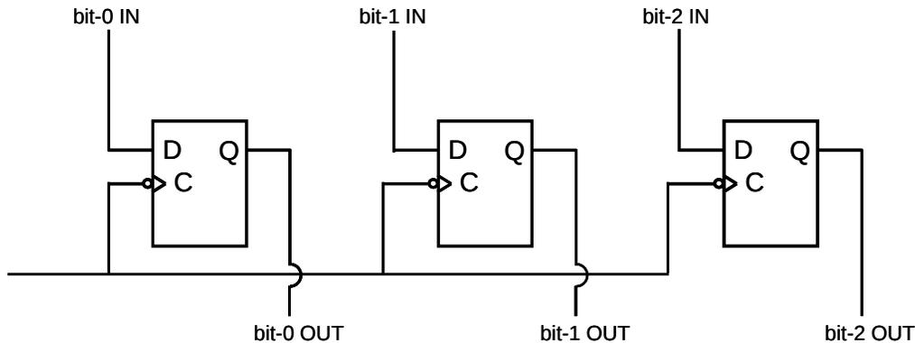
**Figure 4:** Circuit diagram for a 3-bit PIPO-type register.
