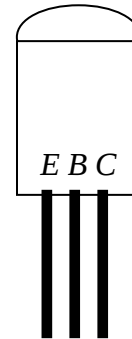
Figure 6.1: A TO-92 transistor package.
