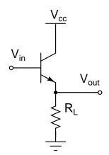
$$V_{out} = V_{in} - 0.6V$$
