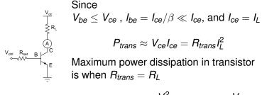
$$max(P_{trans}) = \frac{V_{cc}^2}{4R_L}$$
