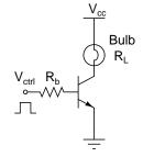
$$I_L = \frac{V_{cc}}{R_L}$$
