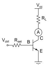
Current through the load resistor does not depend on the load resistance.
