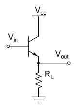
$$V_{out} = V_{in} - 0.6V$$
