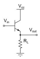
$$V_{out} = V_{in} - 0.6V$$
