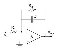
$$G(\omega) = -\frac{Z_c || R_2}{R_1} = -\frac{R_2}{R_1} \frac{1}{1 + i\omega R_2 C}$$
