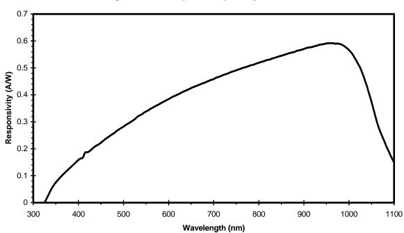
Figure 1 - FDS100 Spectral Responsivity Curve
