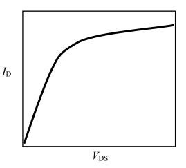
**Figure 8.2**: A sketch of drain current versus channel voltage.
