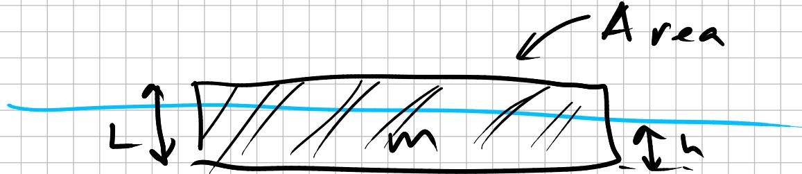
$$m \cdot g = g \cdot \rho_f \cdot V_{\text{submerged}} =$$
