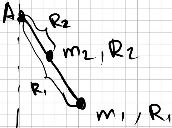
$$E = \underbrace{\frac{m_1 v_1^2}{2} + \frac{m_2 v_2^2}{2}}_K + \underbrace{m_1 j y_1 + m_2 j y_2}_U$$
