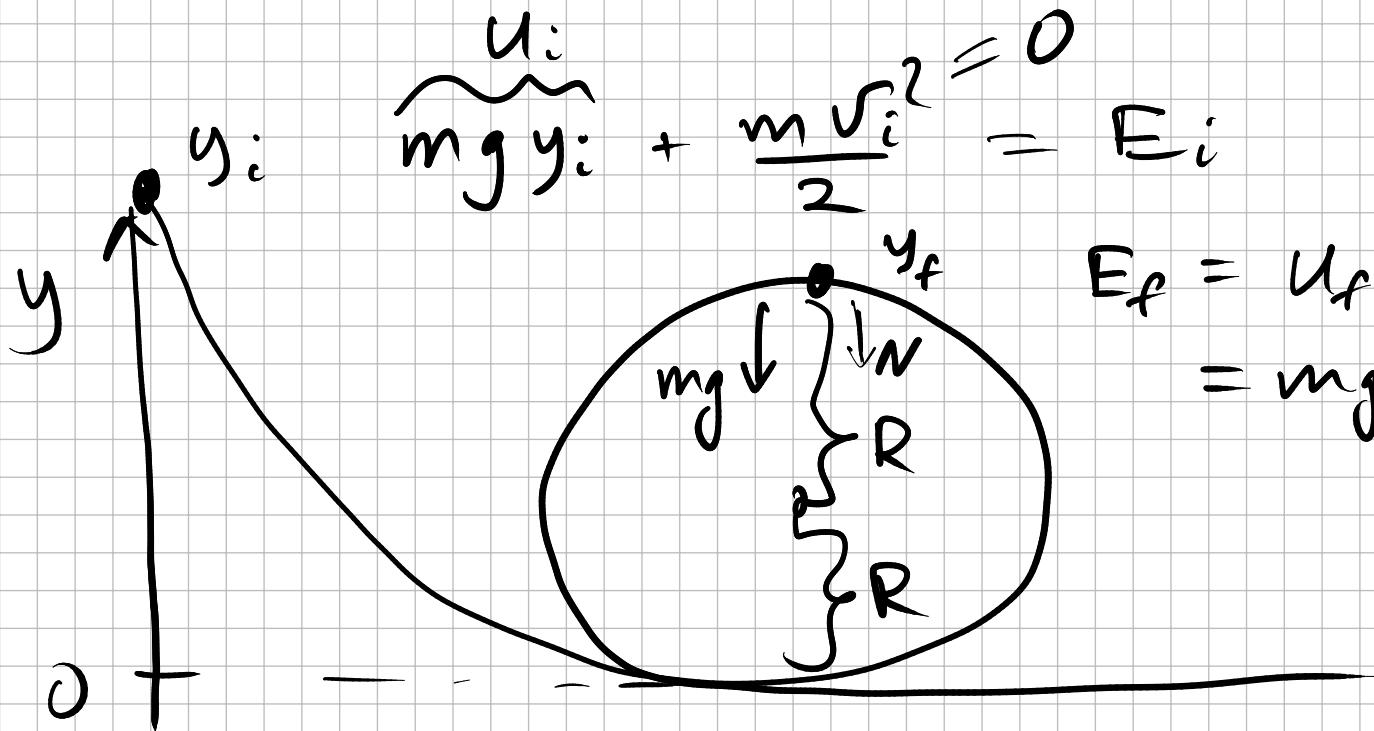
$$\underbrace{U_i}_{mgy_i} + \frac{mv_i^2}{2} = E_i$$
