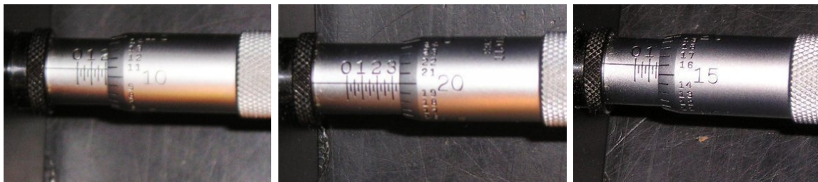
Figure 1.4: Micrometer readings. The coarse division equals to 100 \mu\text{m} , and smallest division on the rotary dial is 1 \mu\text{m} (same as 1 micron). The final measurements is the sum of two. So, from left to right, the figures above show 211 \mu\text{m} , 345 \mu\text{m} , and 166 \mu\text{m} .
