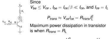
$$max(P_{trans}) = \frac{V_{cc}^2}{4R_L}$$
