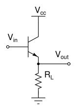
$$V_{out} = V_{in} - 0.6V$$
