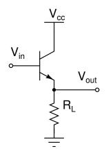
$$V_{out} = V_{in} - 0.6V$$
