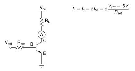
Current through the load resistor does not depend on the load resistance.
