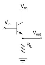
$$V_{out} = V_{in} - 0.6V$$
