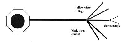
Figure 1.1: The superconducting disk with leads.
