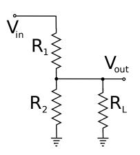
$$egin{aligned} V_{out} &= V_{in} rac{R_2}{R_1 + R_2} rac{R_L}{R_L + R_{1||2}} \ V_{out} &= V_{out_{unloaded}} rac{R_L}{R_L + R_{1||2}} \end{aligned}$$
