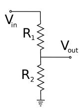
$$V_{out} = V_{in} \frac{R_2}{R_1 + R_2}$$
