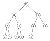
The top most element of the heap is called root.
