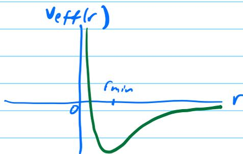
$$r_{\text{min}} = \frac{l(l+1)\hbar^2}{\tilde{Q}^2 \mu}$$
