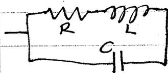
$$Z_R = R, \quad Z_L = i\omega L, \quad Z_C = \frac{1}{i\omega C}$$
