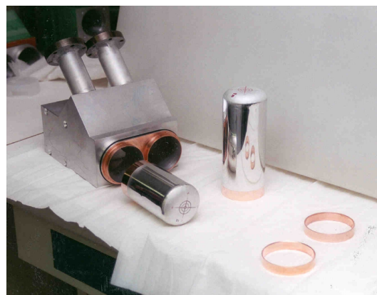
Figure 4.33: Photo of Cell Block and Target Cells. Cell block and target cell cans before assembly.
