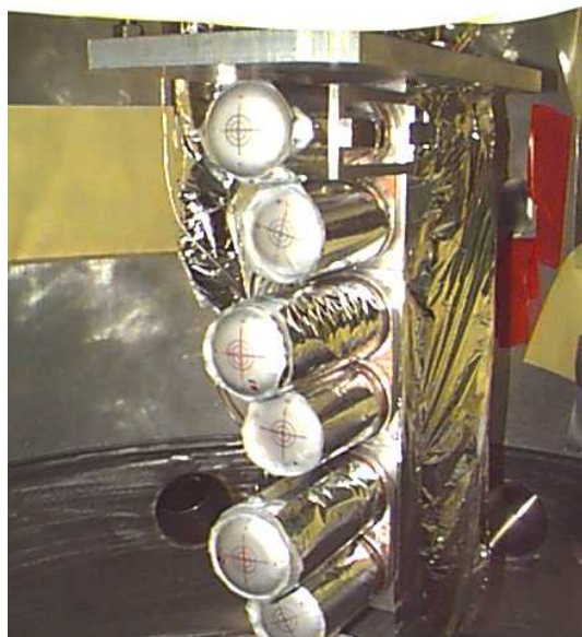
Figure 4.35: Photo of Target Cells. The down-stream 'exit' window can be seen. The cross-hairs on the ends were used in process of measuring the window thickness. The target cells and cell-blocks are wrapped in layers of reflective mylar to reduce thermal radiation and improve cooling efficiency. The Solid target ladder is below the edge of photo.
